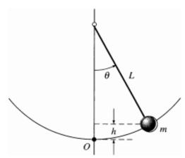
Another example of a mechanical system is given by the **simple pendulum**. In this example we have a mass swinging at the end of a string of length L. We will study the motion of the mass through the counter-clockwise angle  $\theta = \theta(t)$ . Applying the law of the conservation of mechanical energy, which states that the sum of the kinetic and potential remains constant, we will obtain our differential equation.
